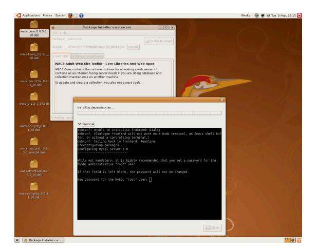
As you can see, it's actually prompting for a new password for the MySQL root user, which we can either enter or just press return to ignore. Generally setting a root password on the MySQL root user is an extremely good idea... With this message acknowledged, the install should actually start making some progress.
